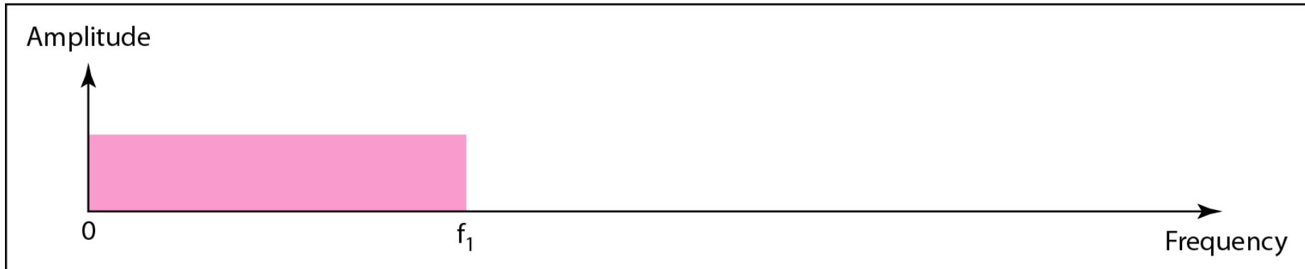
b. Low-pass channel, narrow bandwidth
